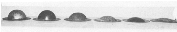
Figure 2 A photograph showing the various stages of formation of the Ti-6Al-4V alloy hemisphere at 950°C. Forming pressure = 0.6 MPa.
