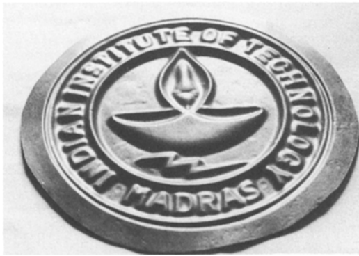
Figure 8 A photograph showing an emblem microformed from the Sn-Pb alloy sheet. Initial thickness = 1.05 mm. Average two-dimensional grain size = 1.2 \pm 0.1 \mu\text{m} . Forming pressure = 0.2 MPa.
